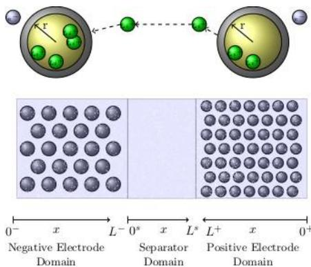
Figure a. Li-ion battery cell EChem representation.
