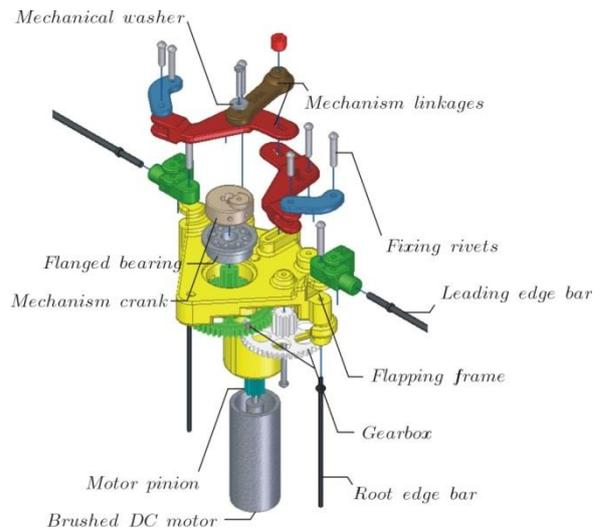
Figure 2: Exploded view of the flapping mechanism.
