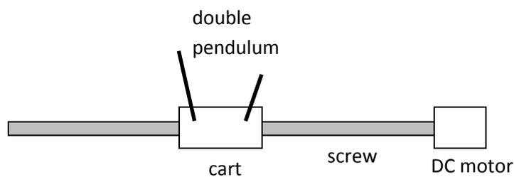
Different sensors are available to measure: the position of the cart and the angles of the two pendulum poles.
