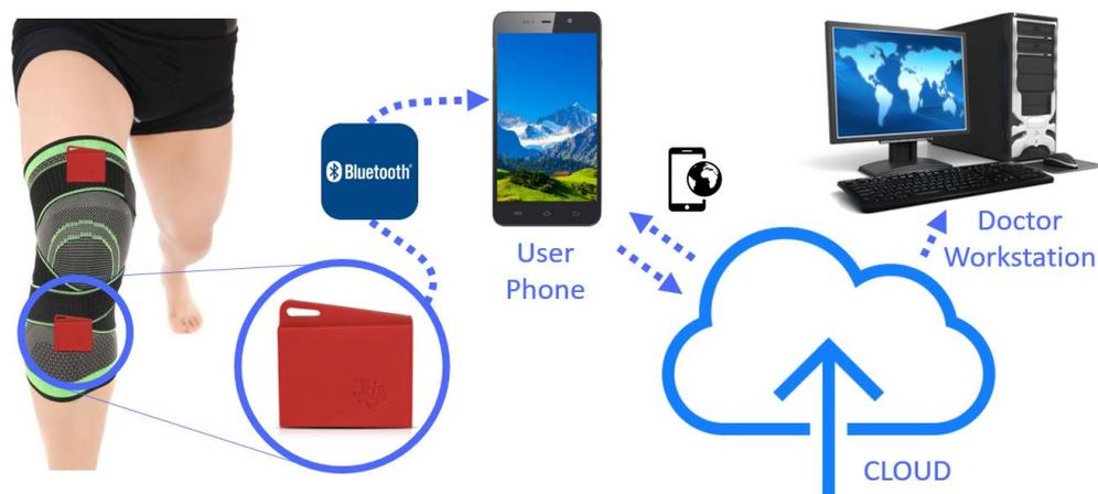
Sensors: 2 TI SimpleLink SensorTags featuring the CC2650 wireless MCU targeting Bluetooth.
